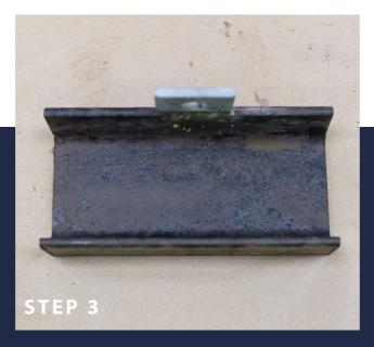
Dramatic colour change from white to navy/black shows that the rust has been effectively neutralised. Wipe surface to remove any residue.
