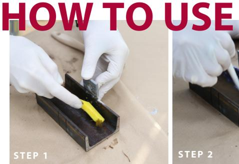
Clean and degrease using suitable HMG Prep Clean.
