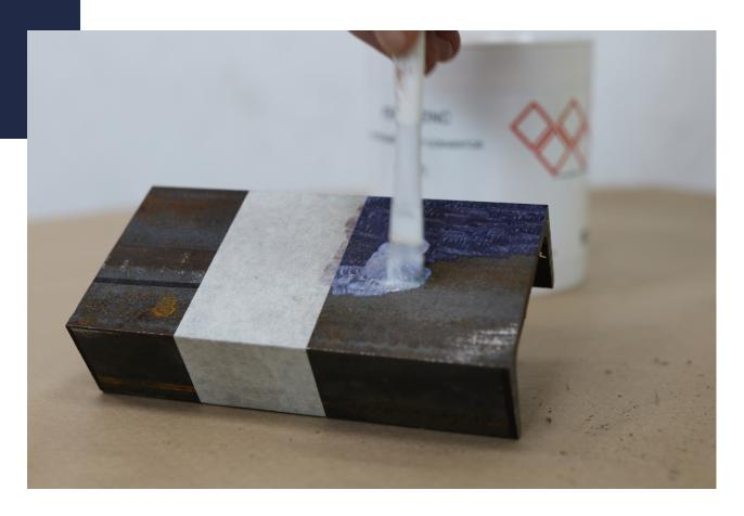
Ideal for structural steel, fences, iron railings, guttering, external ferrous metals, vehicle and machinery and marine situations due to application to damp surfaces that are difficult to completely dry e.g. light condensation or surface moisture, not for application during wet weather.
